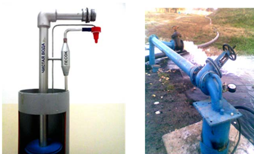
Figure 3 – The types of the end walls of the well with minimization – thickener (a) and work well with purified water (b)
